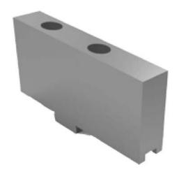
FWB soft jaws are used for precision gripping of previously machined workpieces which must not be damaged on the gripped surface. These jaws are suitable for light cutting and are turned and ground to suit the shape of the workpiece in the chuck under gripping force. Turned FWB top jaws maintain their precision as long as they are not removed from the base jaw they were ground in.
