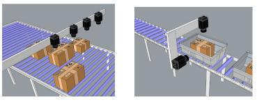
To configure multi-reader triggering, select the **Master/Slave** pane in the Setup Tool (under **System Settings**). For more information, see the *DataMan Fixed Mount Readers Reference*.
