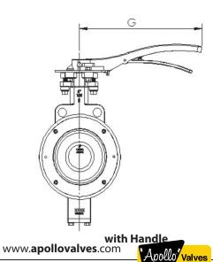
handle & gear dimensions - fire safe & metal seat
