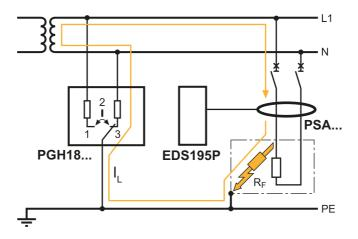
Abb. 4.1: EDS operating principle
