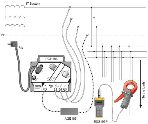
Abb. 6.3: Connection diagram EDS309... with AGE185
