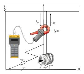
Abb. 3.2: Part of the current flows through an insulation fault  $R_F$  The sum of the two currents is no longer zero. As soon as the residual current reaches or exceeds the response value there is an alarm message on the EDS195P.
