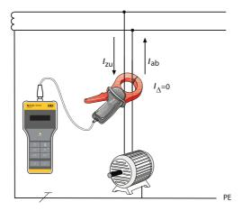
Abb. 3.1: The two currents  $I_{zu}$  and  $I_{ab}$  have the same magnitude, however their signs are different, such that the sum of the two currents is zero. The EDS195P detects this situation, there is no message.
