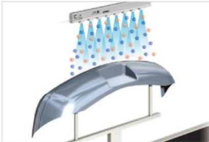
Static elimination in the coating process of bumpers
