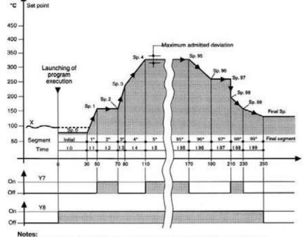
Fig. 5: Example of Programmed Set point with priority slope.
