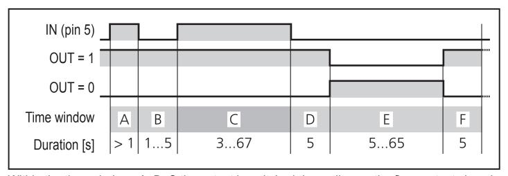
Within the time windows A, B, C the output is switched depending on the flow: output closed (OUT = 1) if flow  $\geq$  SP / output open (OUT = 0) if flow  $\leq$  SP.
