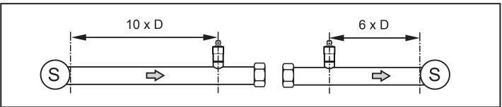
D = pipe diameter; S = sources of interference
