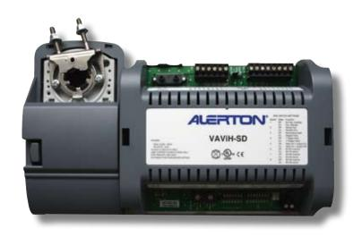
The Alerton BACtalk® VAViH-SD™ controller with integrated actuator is a versatile BACnet-compliant controller, providing pressure-independent control of any single-duct variable air volume (VAV) box. It features a built-in airflow sensor, five universal inputs (Als or BIs) and six binary outputs (BOs). As a native BACnet controller, the VAViH-SD integrates seamlessly with your BACnet system, communicating at up to 76.8 Kbps on a BACnet MS/TP LAN.
