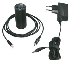
The combined Read-out Head K01-Blue is used in combination with a PDA/PC with Bluetooth functionality for optical read-out of devices with interface according to IEC 62 056-21 (IEC 1107). In addition, the device is equipped with a CS/CL interface.
