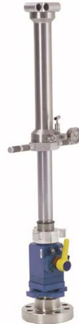
Once the service valve has been closed and the retriever is isolated from the process pressure, the bleed valve then allows the product inside the retriever to be bled away for safety and cleanliness. It also can be used for product sampling and is required for use when back pressuring.
