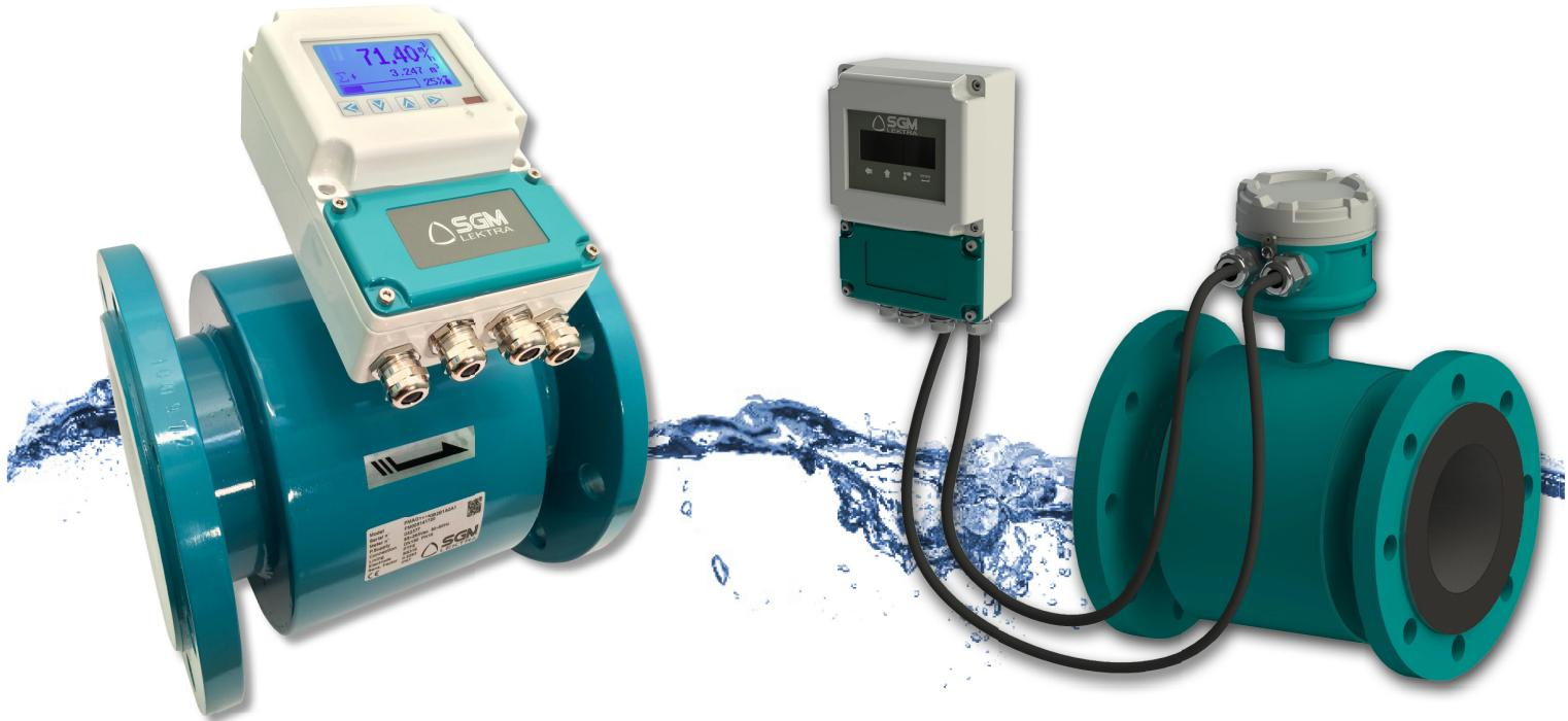
Pmag flowmeters are particularly suitable for all types of wastewater measurements. A various types of lining material are available to suit chemically aggressive liquids or with suspended solids. A salient feature of the soft rubber lining is the resistance to abrasion due to water with suspended solids.
